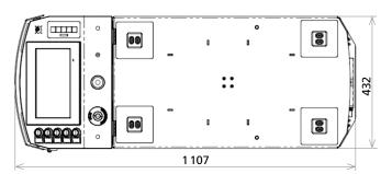
AGV/AMRs are designed exactly to the needs of a given customer's application. AGV/AMR RoboCaddy II can be equipped with a robot, roller conveyor, belt conveyor or other superstructure.
